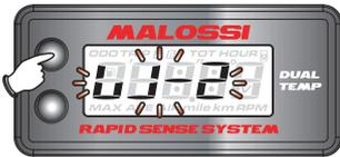
• Press the **upper button** to enter the overheat temp B warning setting.
