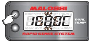
• Press the **upper button** to return to the overheat temp B warning setting.
