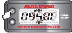
• Press the **upper button** to return to the overheat temp A warning setting.
