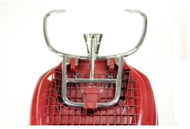
To attach the top case to the carrier you need to drill a hole in the top case and use the 605339M mounting kit.
